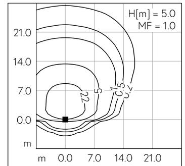
LED 3000 K 69 W 9978 lm-h H = 5 m / CIE Flux 31 69 95 100 100 / A20 selon DIN 5...
