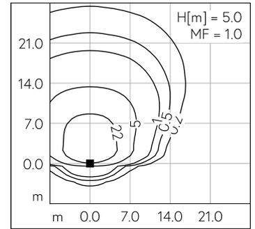
LED 3000 K 34.5 W 4989 lm-h H = 5 m / CIE Flux 31 69 95 100 100 / A20 selon DIN...
