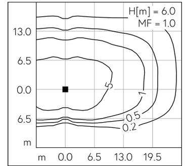
LED 3000 K 52.2 W 7170 lm-h H = 6 m / CIE Flux 38 75 96 100 100 / A30 selon DIN ...
