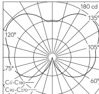
LED 4000 K 18 W 1829 lm-h 272°/272° / CIE Flux 11 35 65 40 100 / C12 selon DIN 5...
