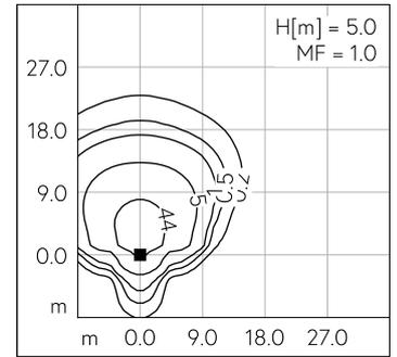
LED 4000 K 58.5 W 7160 lm-h H = 5 m / CIE Flux 39 80 99 100 100 / A30 selon DIN...
