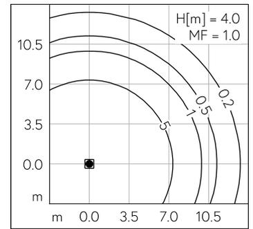
LED 4000 K 26 W 2271 lm-h H = 4 m / CIE Flux 19 73 98 99 100 / A10 selon DIN 5040
