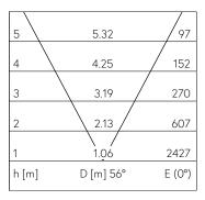
LED 3000 K 30 W 2960 lm-h 56° / CIE Flux 0 0 0 0 100 / E84 selon DIN 5040
