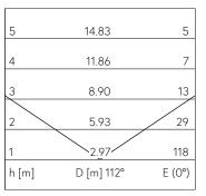
LED 3000 K 4.8 W 332 lm-h 110°/112° / CIE Flux 0 0 0 0 100 / E83 selon DIN 5040
