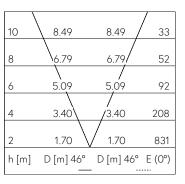
LED 3000 K 35.3 W 3292 lm-h / CIE Flux 0 0 0 0 100 / E84 selon DIN 5040
