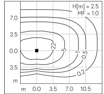
LED 4000 K 31 W 4218 lm-h H = 2.5 m / CIE Flux 41 77 96 100 100 / A30 selon DIN ...
