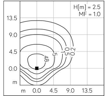
LED 4000 K 22 W 2661 lm-h H = 3 m / CIE Flux 39 81 97 100 100 / A30 selon DIN 5...
