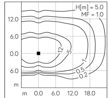
LED 4000 K 69 W 9764 lm-h H = 5 m / CIE Flux 38 75 96 100 100 / A30 selon DIN 5...
