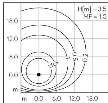
LED 4000 K 39.7 W 3212 lm-h H = 3.5 m / CIE Flux 41 74 93 92 100 / A31 selon DIN 5...
