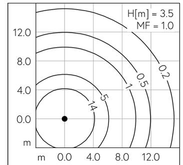
LED 4000 K 39.7 W 3212 lm-h H = 3.5 m/ CIE Flux 41 74 93 92 100 / A31 selon DIN ...
