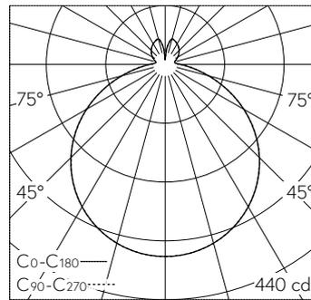
LED 3000 K 13.3 W 1285 lm-h / CIE Flux 45 75 92 86 100 / B42 selon DIN 5040
