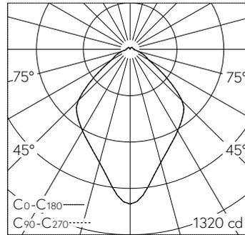
LED 2700 K 19.5 W 1998 lm-h / CIE Flux 59 88 97 94 100 / A51 selon DIN 5040
