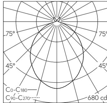
LED 3000 K 13.5 W 1389 lm-h / CIE Flux 54 85 97 90 100 / A53 selon DIN 5040
