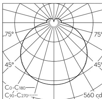
LED 3000 K 18.6 W 1865 lm-h / CIE Flux 41 70 90 84 100 / B31 selon DIN 5040
