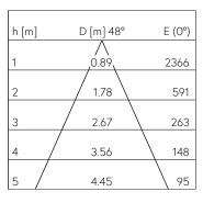
LED 3000 K 27.9 W 1365 lm-h 48° / CIE Flux 98 100 100 100 100 / A80 selon DIN 5...
